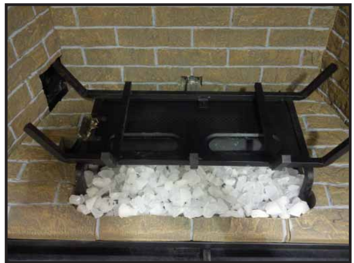
Figure 11.9. Ember Glass Area Covered with Teco-Sil
