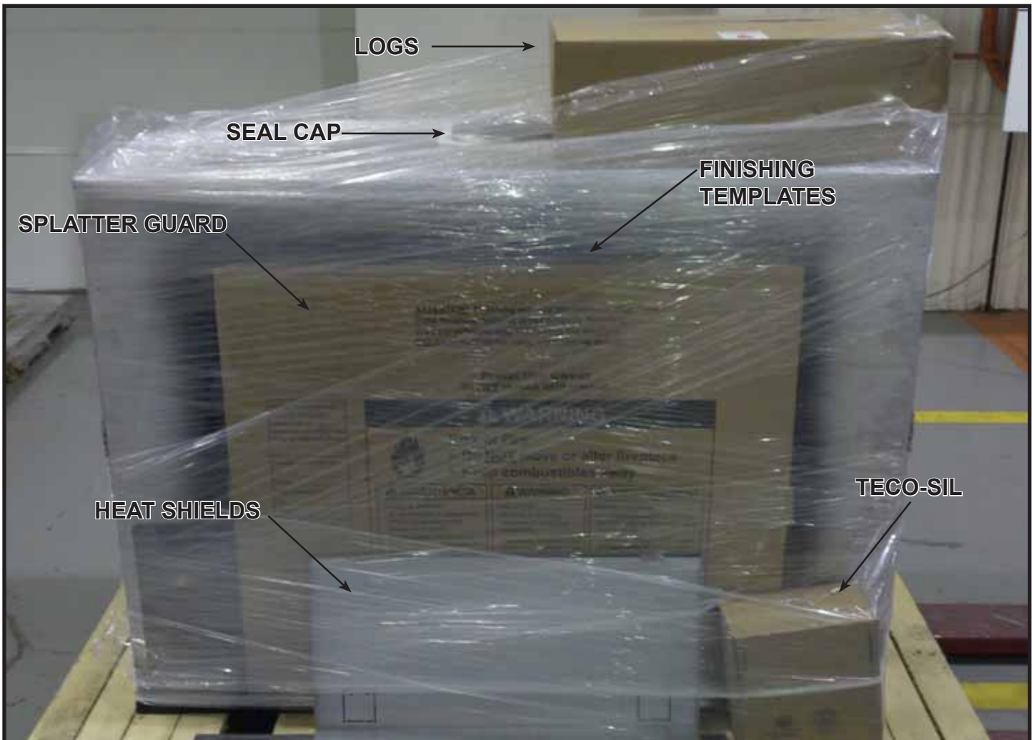
Figure 6.1 Shipping Location of Components
