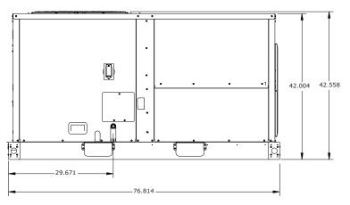
NOTES: 1. THRU-THE-BASE GAS AND ELECTRICAL IS NOT STANDARD ON ALL UNITS. 2. VERIFY WEIGHT, CONNECTION, AND ALL DIMENSION WITH INSTALLER DOCUMENTS BEFORE INSTALLATION.
