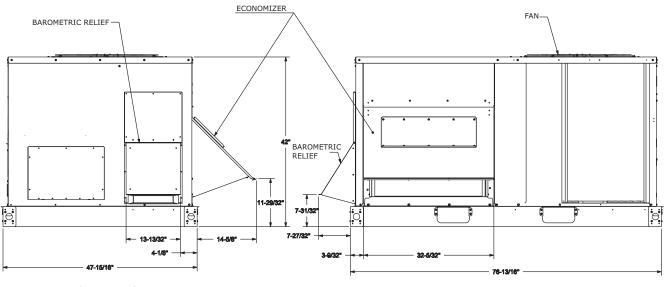
Figure 8. Barometric relief and economizer – 3–5 tons
