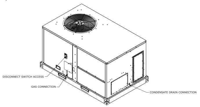
Figure 3. Gas/electric units - front & side views - 3-5 tons
