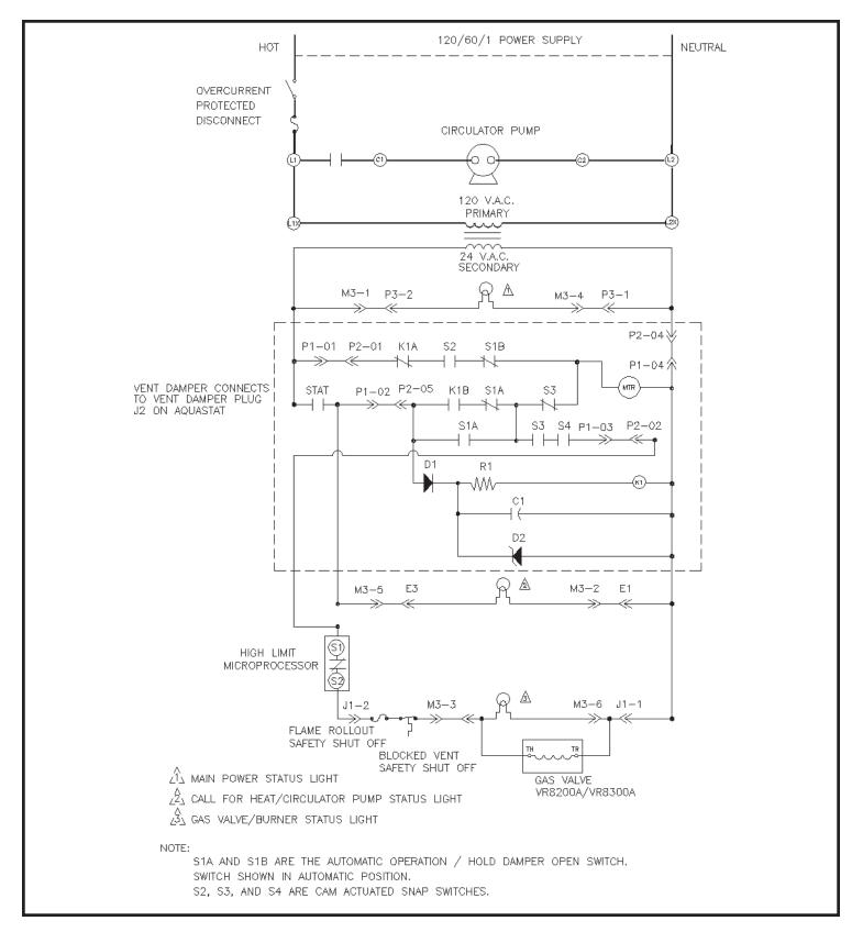
IF ANY OF THE ORIGINAL WIRE AS SUPPLIED WITH THIS APPLIANCE MUST BE REPLACED, IT MUST BE REPLACED WITH TYPE 105° C THERMOPLASTIC WIRE OR IT'S EQUIVALENT
