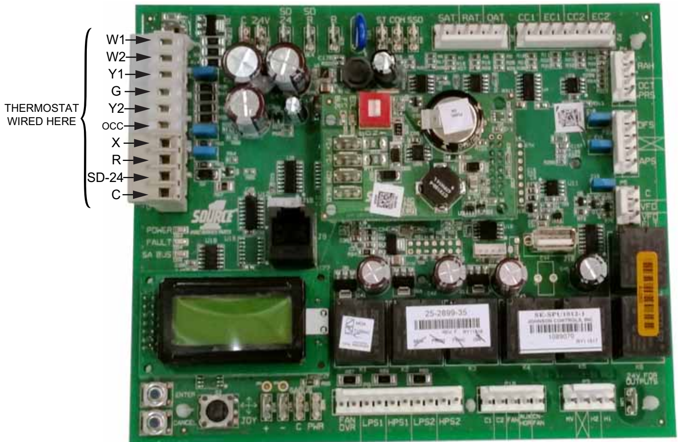
Figure 20: Unit Control Board
