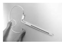
Above — Use Series 1227 as a regular U-tube manometer to read high-range pressure on the right leg, or as an inclined manometer (shown here) to read low-range pressure on the bottom leg. Simply incline manometer until fluid levels read zero. No spirit level required. Magnetic clips hold the gage in position on a steel duct surface.
