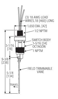
psig (10 bar) and temperatures to 212°F (100°C). The V8 flow switch can be used in various chemical processes, industrial systems and similar applications where process conditions are compatible with polyphenylene sulfide, ceramic 8 and 316SS. The V8 Flotect® flow switch is UL recognized as an industrial motor controller per UL standard 508, suitable for mounting in a protected environment.
