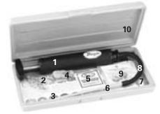
Easy-to-Use Smoke Gage Kit enables you to quickly balance maximum  $CO_2$ with minimum smoke for clean, efficient combustion. Simply take an actual sample of the smoke being tested and compare it to the standards on the Smoke Chart included. Just 10 full strokes of the pump produces an accurate test sample. Complete testing instructions are included.
