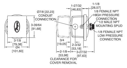
Construction and dimensions. Series 1823 pressure switches.
