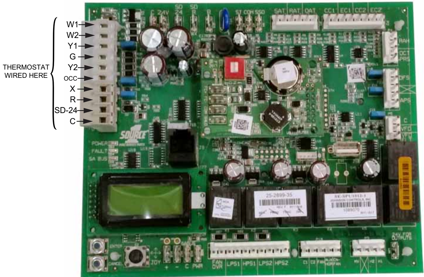
Figure 35: Unit Control Board
