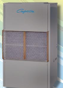
These individual packaged units transfer heat via water loop systems for effective heating and cooling. Our largest capacity units, they feature belt drive blowers and reliable scroll compressors. Power and water connections can be made on either side (also refrigerant connections for HKV), and discharge air is field convertible.
