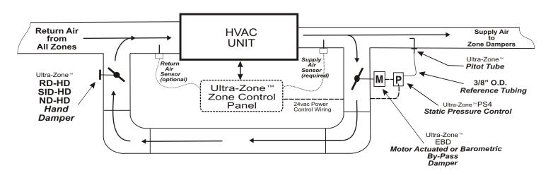
Note: This drawing of the Bypass damper static pressure control and related duct work is intended to serve only as a guide, your actual duct work layout may differ substantially.
