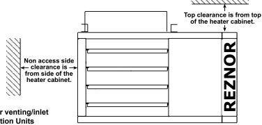
Refer to Reznor web site www.RezSpec.com for venting/inlet air requirements for Reznor Separated Combustion Units
