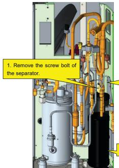
2. Remove the screw bolt of the separator.
