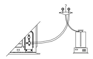
4. Keep the refrigerant tank erect and put it on an electronic scale. Zero the scale.
