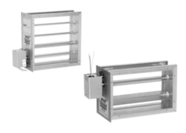
The ZD is a power close and spring open damper. It has a 24-volt motor used to control circulating air in heating, cooling and ventilating systems. It is used when a normally-open damper is required. The ZD is typically used with the TrueZONE systems and other electronic zoning systems.
