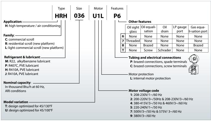
Version T compressors are built with a threaded oil equalization port to be used with our variable speed compressors range VZH.
