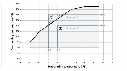
**Example 1** (R410A, SH =  $20^{\circ}$ F) LP switch setting: LP1 = 60 psig ( $0^{\circ}$ C) HP switch setting: HP1 = 550 psig ( $140^{\circ}$ F) ① The LP and HP switches don't protect sufficiently from operation outside the envelope. A DGT protection is required to avoid operation in the hatched area.
