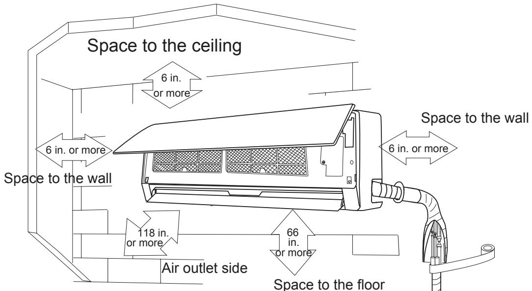
The dimensions of the space necessary for correct installation of the appliance including the minimum permissible distances to adjacent structures
