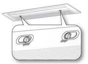
Push the [PUSH] tabs located in 3 places to unlock the groove on the front grille.
