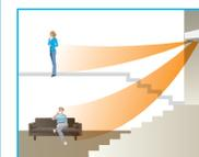
Our double vane separates the airflow in the left and right directions to deliver airflow not only across a wide area of the room, but also simultaneously to two people in different locations.
