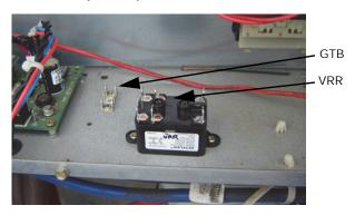
**Note:** For multispeed conversion the second relay (VSR) would be installed to the right of the VRR pictured.
