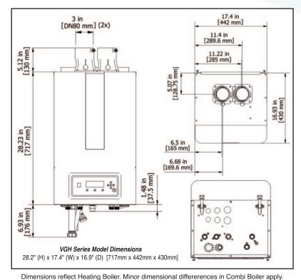
Our VGH Residential Series boasts 95% efficiency, with a a stainless steel heat exchanger for durability, superior heating and corrosion resistance with an easy to use control that spans the entire VGH product family from residential to commercial.
