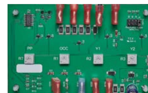
“V” Vent Control Board
