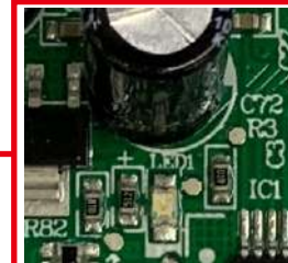
LED1: Drive failure indicator
