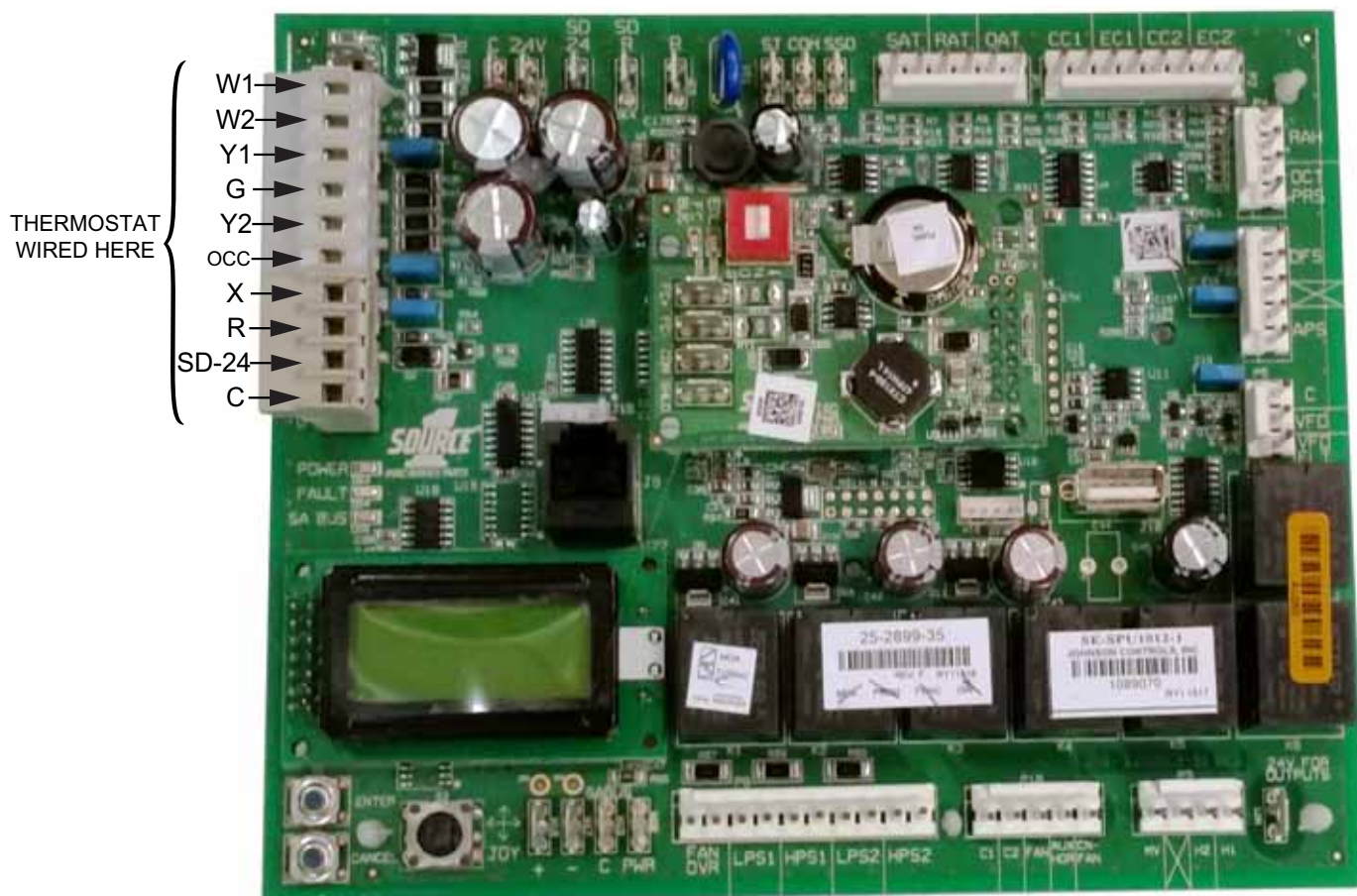
Figure 15: Unit Control Board
