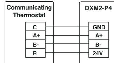
**Note:** Order chassis for communicating thermostat or field rewire.
