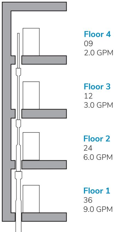
**Unit GPM (UGPM)** = Required gallons per minute from "Performance Charts," or GPM used to calculate unit capacity.
