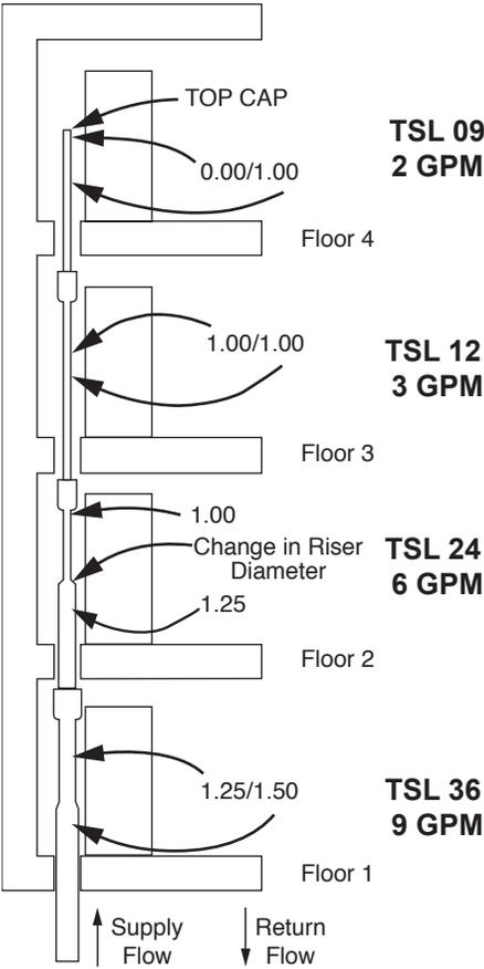
From Table 1 (below) determine the proper riser diameter needed to satisfy the required GPM's at each unit. Refer to Table 2 (below) for a summary.
