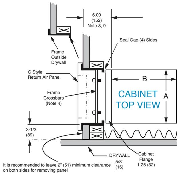
It is recommended to leave 2" (51) minimum clearance on both sides for removing panel
