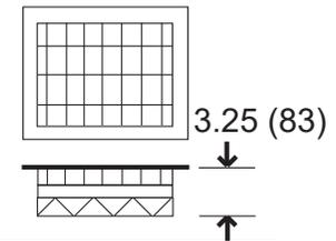
**Unequal Air Flow** - Air discharges requiring different air volumes (CFM). Use double deflection with opposed blade damper grilles.
