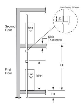
**Riser Extension Length:** Start with the floor to floor Dim. (FF) From this subtract the room riser height and tail length. Then add 4" (102) for the two joint overlaps.
