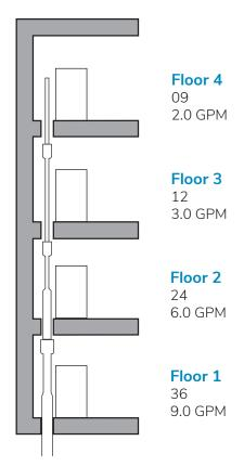
**Unit GPM (UGPM)** = Required gallons per minute from "Performance Charts," or GPM used to calculate unit capacity.
