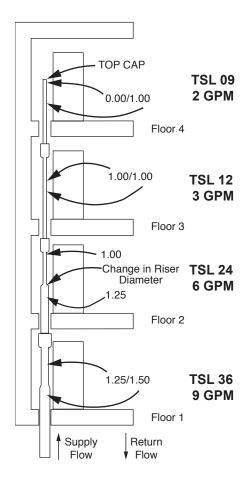
From Table 1 (below) determine the proper riser diameter needed to satisfy the required GPM's at each unit. Refer to Table 2 (below) for a summary.
