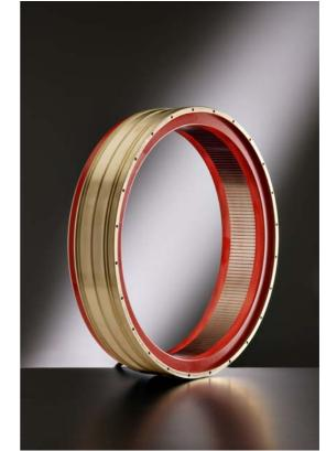
All TK motors are designed for fluid (water) cooling on the outside of the stator for maximum performance. Conduction/convection cooling is also possible. Constant power operation (flux control) always requires water cooling.
