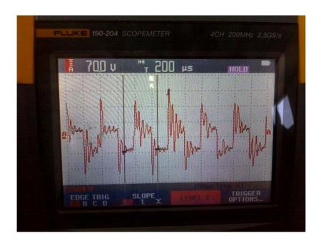
To prevent such resonance, Phase supplies with each motor with such characteristics a tuned anti resonance filter (snubber) which must be assembled within 5 m of the motors, between the motor star terminal (white wire) and machine ground. Failure to connect the snubber may result in motor failure by insulator puncturing.
