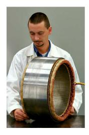
A three phase stator, wound and impregnated (3 dips, preferred solution for high thermal cycling), or vacuum encapsulated in super high thermal conductivity compound (for low surface temperature operation), which is either built into a thin steel microframe, cylindrical, or into a metallic frame carrying the cooling chambers and coupling O-Rings on the outside and a set of tapped holes on one side (Squid type).
